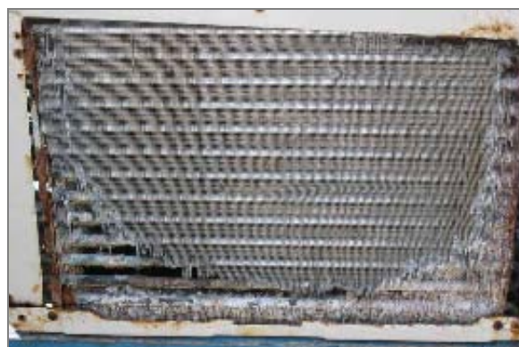
Inefficient badly corroded heat exchangers are very common in Majuro's air conditioners
